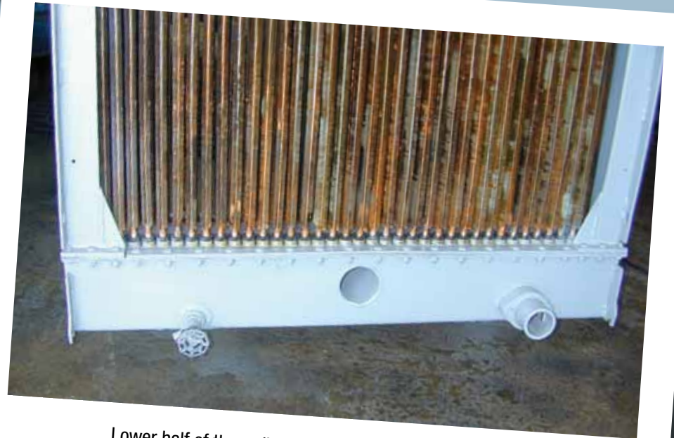
Lower half of the radiator showing a lot of discoloration, but tubes in good enough shape to keep on working.
